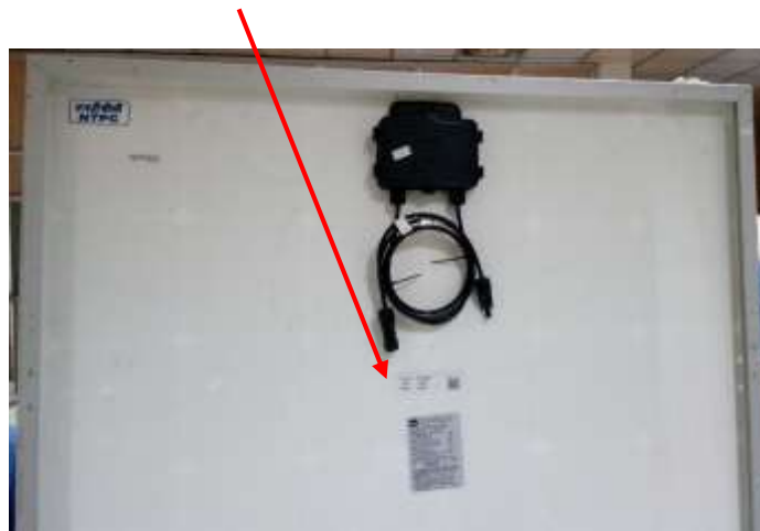
RFID Tag position outside the laminate
